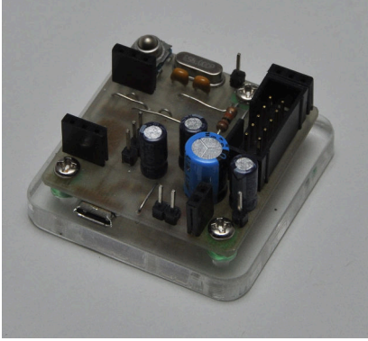
(a) Transmitter module consisting of a microcontroller, a voltage doubler and H-Bridge power amplifier (without ultrasonic transmitters).
