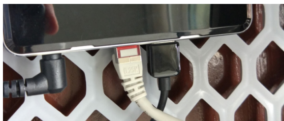
Figure 4.1: Loose contacts of a network cable (white)
